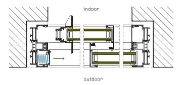
Horizontal section 1:5 Side wall fixture, open insect screen
