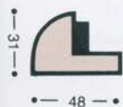
2112T DOOR STOP • floor mounted • particularly suitable for use with deep pile carpets or stepped thresholds
