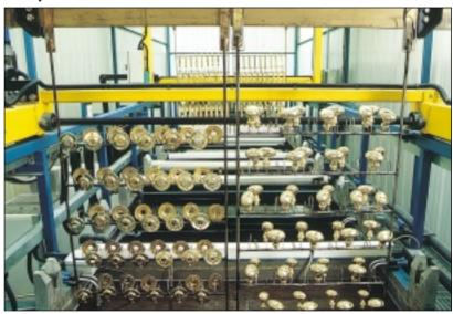
Polished brass door knobs and roses moving along Frank Allart's automated and computer controlled electrophoretic lacquering plant.
